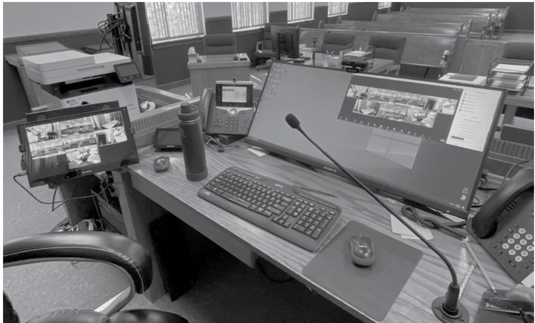
Video setup consists of five webcams and four microphones. The courtroom gallery camera utilizes an AV cart adjacent to the bench, with a large TV and small PC. The remaining four cameras — one at each counsel table, one on the bench, and one in the witness box — are hooked to small PCs.
